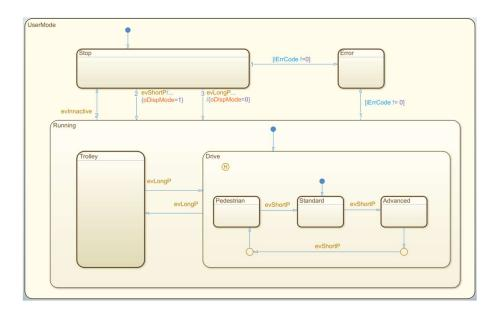
The events identified as "evShortP" and "evLongP" correspond to the short and long press of the configuration button. Note that the keypad action is inhibited when the vehicle is in motion. Therefore the change is permitted even if the vehicle is stationary.
